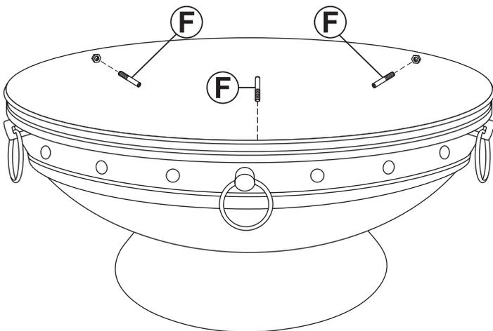
Hand-tighten three M8x25mm Grub Screws (F) to the inside rim of the fire-bowl.
