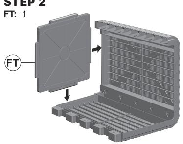
Insert Bottom Panel (FT) into the bottom of one of the assembled side panel sections, as shown.
