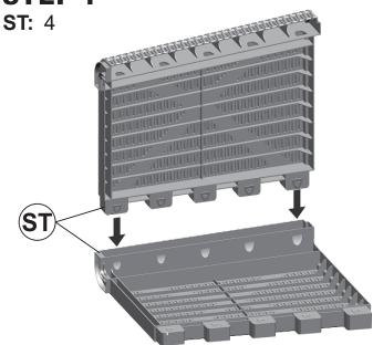
Firmly press the straight side of one Side Panel (ST) into the rounded side of the second Side Panel, as shown. Repeat with the remaining two side panels.
