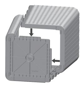
As shown, align the remaining assembled side panel section with the bottom panel.
