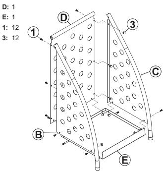
Align Back Panel (D), Left Panel (B), and Right Panel (C), on the inside of Bottom Panel (D) and loosely secure all components using M6x10mm Bolts (1) and Cap Nuts (3).
