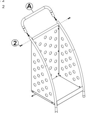
Insert Handle (A) into the side panels and secure using M6x30mm Bolts (2).
