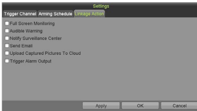
Figure 8-10 Alarm Linkage Actions
