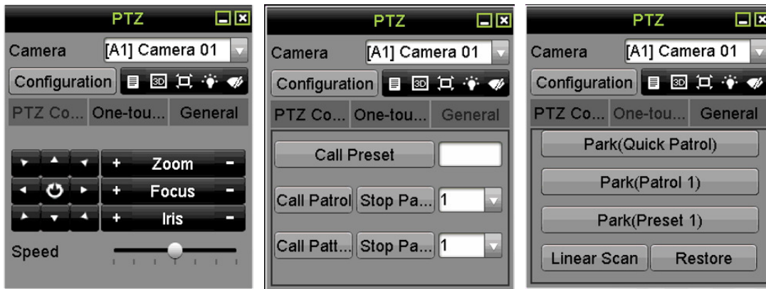
Figure 4-14 PTZ Control Panels
