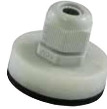
**DC-01) Duct collar** - The DC-01 is an adjustable collar for mounting the duct temperature sensor probes. It incorporates a foam backed mounting flange with 2 mounting holes. A compression type fitting accommodates a 1/4" probe and allows for an adjustable probe depth.
