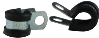
**TS17R-\*) Probe clamp** – The TS17R-\* is a zinc plated, rubber coated tube clamp that can be used to secure a temperature probe. It is available in several sizes to fit a wide variety of probes.
