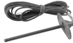
**C & AP) Immersion Sensor** – The C comes in two configurations. It has either spring loaded or non-spring loaded probes and has a 1/2" NPT fitting to be mounted into a thermowell. It is available in various lengths and enclosure styles. The AP is a non-spring loaded probe with a 1/2" NPT fitting to be mounted in a thermowell.
