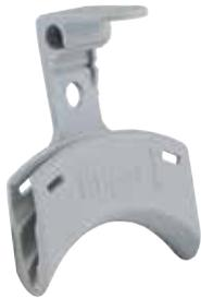
**CC-1G) Averaging probe clip** – The CC-1G is used to mount averaging sensors in duct applications. It can be used for probe diameters of 1/8", 1/4" and 3/8". The bracket provides support and a smooth arc for direction reversal allowing for criss-crossing the duct. It eliminates kinking of the sensor and damaging the probe.
