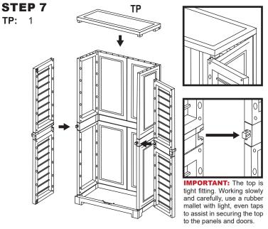
Affix the backside of Top Panel (TP) to the back and side panels; do not affix the front of the top panel.
