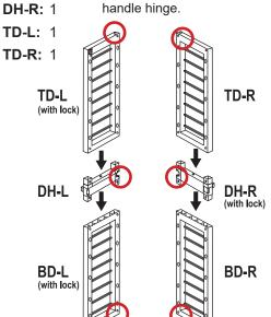
Assemble the doors as shown: Top door, handle, bottom door.
