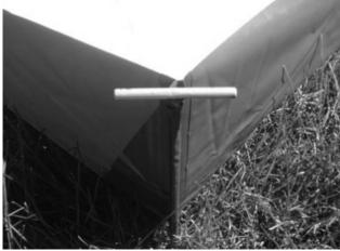
4. Clip the pivoting side support brackets in the punched holes around the perimeter of the liner.
