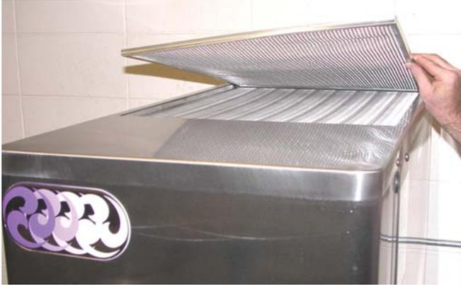
Figure 4-4 Removing Condenser Filter
