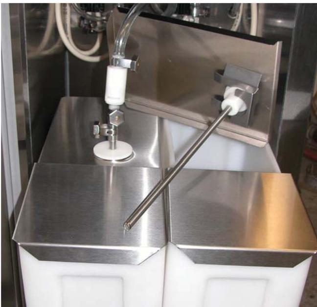
Figure 2-5 Connecting Mix Pick-up Assembly
