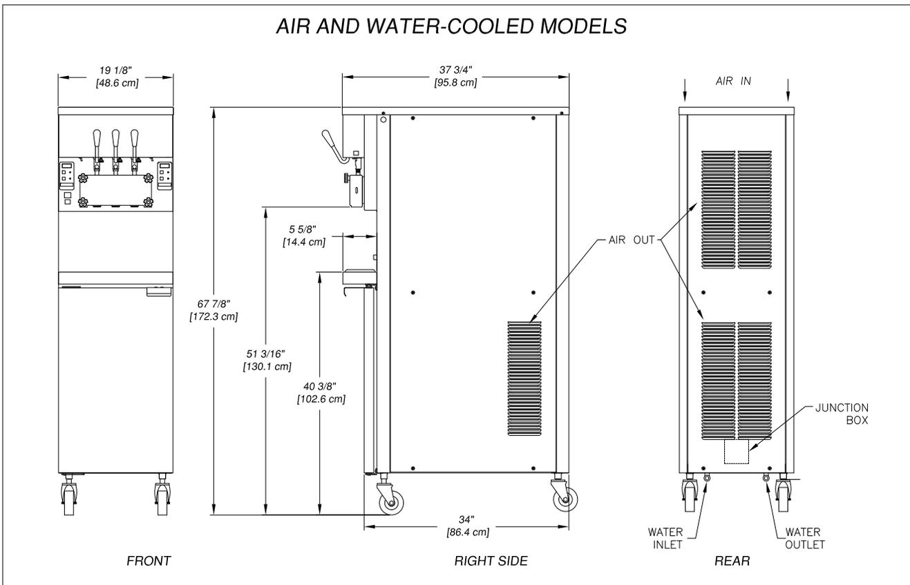
**Figure 1-2 Machine Specifications**
