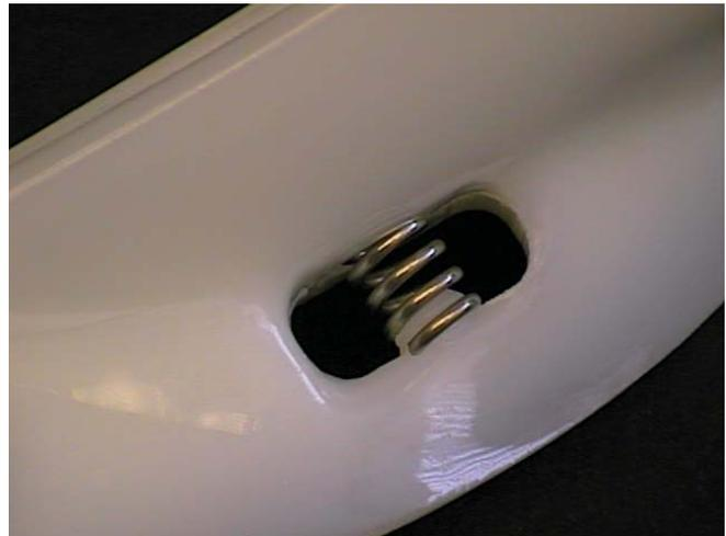
**Figure 3-8 Spring Installation**
