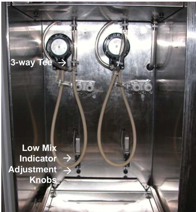
**Figure 2-6 Connecting Pump Hose to BCS Manifold**
