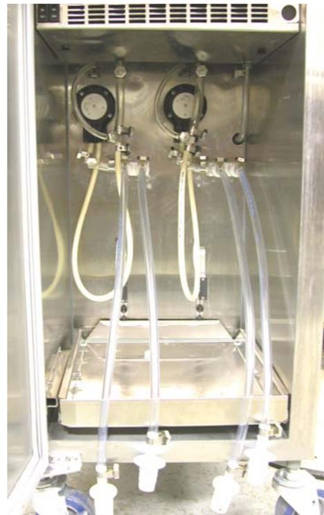
**Figure 2-7 Completed BCS Hose Assembly**
