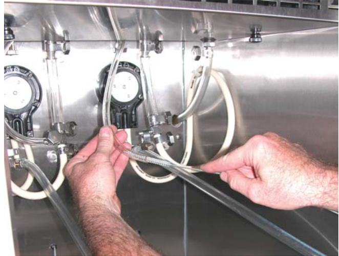
**Figure 3-18 Cleaning Air Tube**
