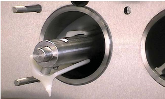
**Figure 3-5 Auger Flight Removal**
