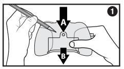
1. Press down on release button (A) to slide down battery cover (B).
