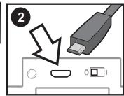
2. Plug the small end of the charging cable into the charging port.
