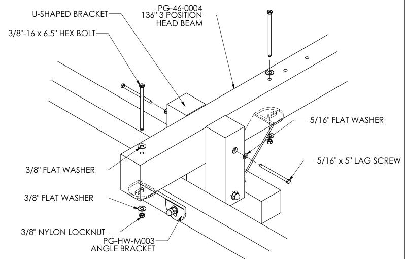
(Prop up the end of Head Beam 6" for it to lay flat in the U-Shaped Bracket)
