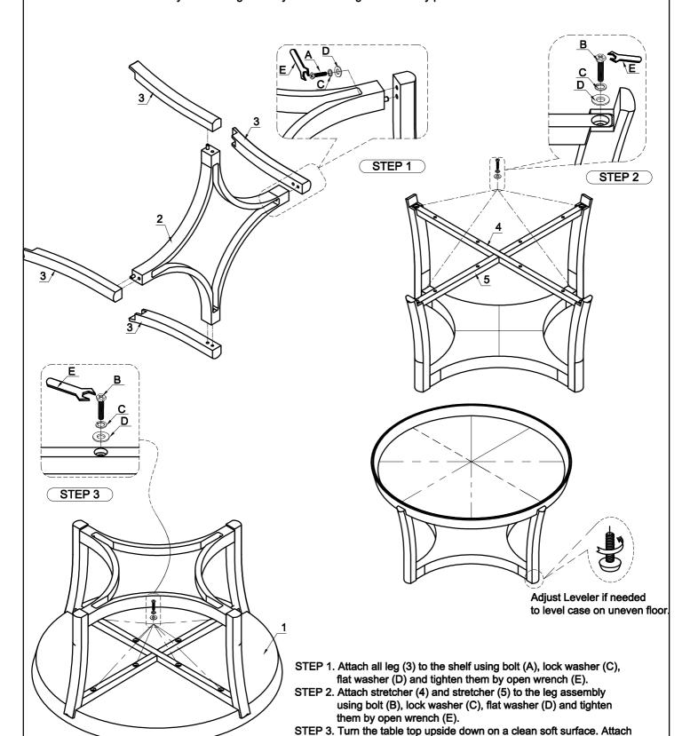
the leg assembly to the table top using bolt (B), lock washer (C), flat washer (D) and tighten them by open wrench (E).
