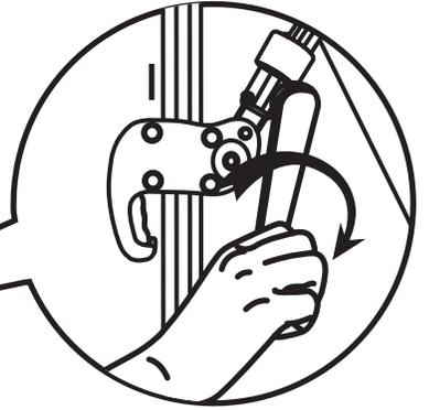
Bottom Crank Hole for 360 degree rotation
