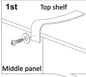
Drill your wall with a 6mm drill (not included) and insert bush, securing wall anchor gift washer and screw in the wall.
