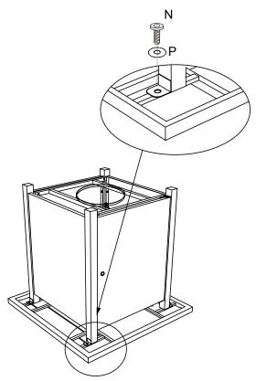
Step4.Attach the assembled base to the bottom of top using 4pcs of screws (N),and 4pcs M6 washers(P), make sure the panel (L) faces the valve stem. Tighten all screws.
