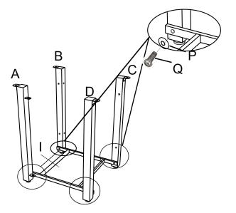
Step1.Connect the tank holder/base (I) With table Lets(A/B/C/ D) by 4pcs screws (Q)and 4pcs M6 washers(P).
