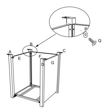
Step2. Connect panel (E,F,G)with table legs(A,B,C,D) by 12pcs screws (Q) and 12pcs M6 washers(P).
