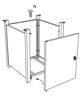
Step3.Hang the bottom (H) of the door plate on the round bracket.Top with 1PC screw(N)lock.
