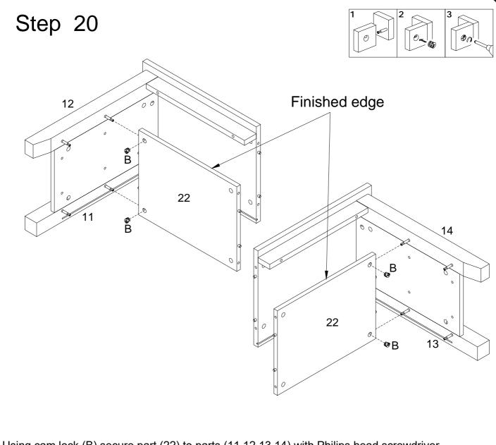
Using cam lock (B) secure part (22) to parts (11,12,13,14) with Philips head screwdriver as per diagram.
