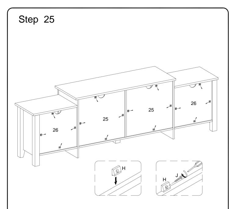
Using screw (J) secure plastic wedge (H) to parts (25,26) with Philips head screwdriver as per diagram.
