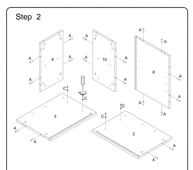
Insert wooden dowel (A) into parts (2,3,6,8,10) ,then secure cam bolt (C) into parts (2,3) with Philips head screwdriver as per diagram.
