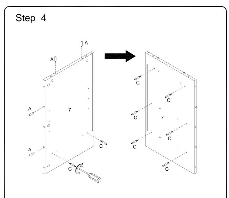
Insert wooden dowel (A) into part (7), then secure cam bolt (C) into part (7) with Philips head screwdriver as per diagram.
