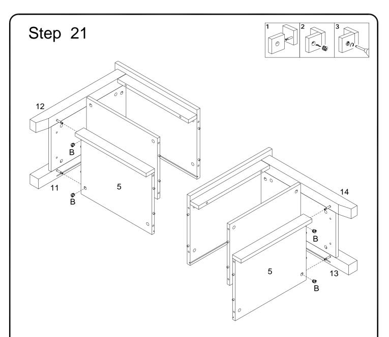
Using cam lock (B) secure part (5) to part (11,12,13,14) with Philips head screwdriver as per diagram.
