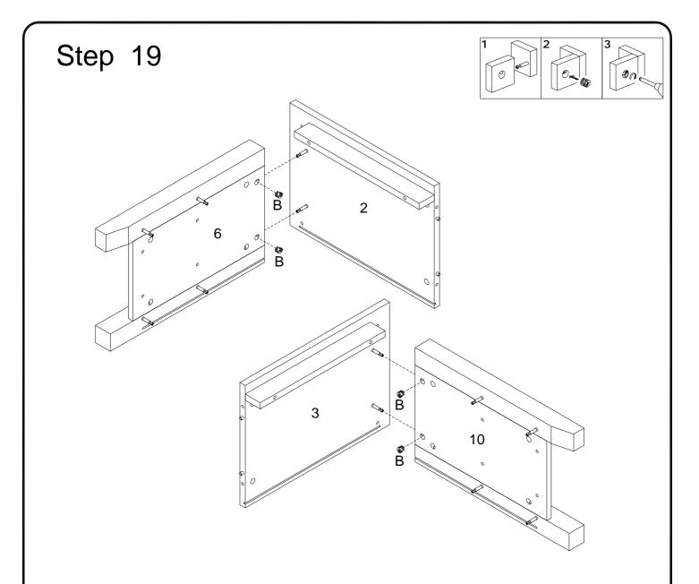
Using cam lock (B) secure part (6) to part (2) ,part (10) to part (3) with Philips head screwdriver as per diagram.
