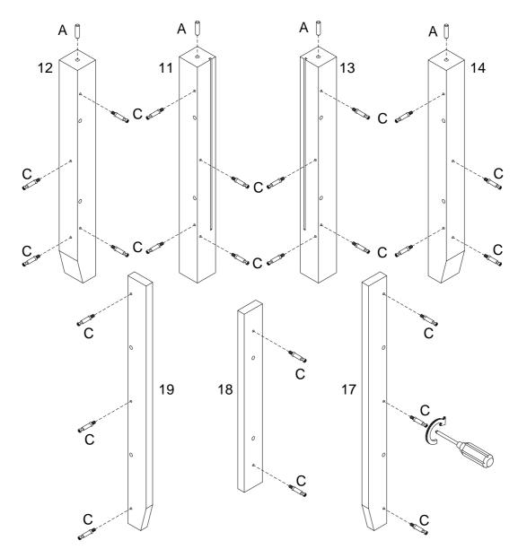
Insert wooden dowel (A) into parts (11,12,13,14) ,then secure Cam bolt (C) into parts (11,12,13,14,17,18,19) with Philips head screwdriver as per diagram.
