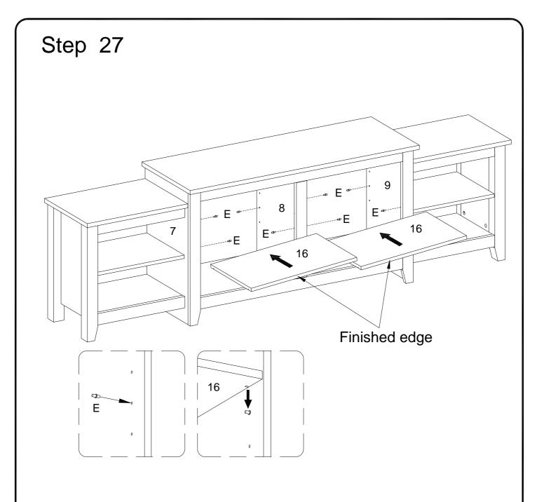
Insert shelf support pin (E) into parts (7,8,9) as per diagram. Make sure you place the shelf support pins (E) in the same level. So the shelf is not titled .Put part (16) into unit as per diagram. Tilt and rest the adjustable shelf(16) onto the shelf support pins .
