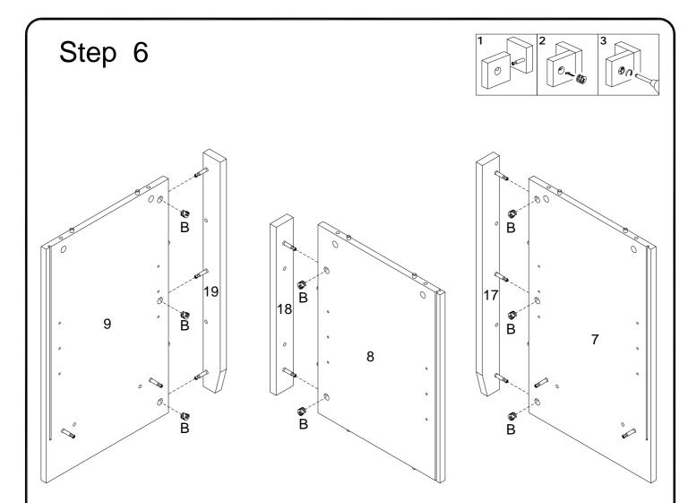
Using Cam lock(B) secure parts (17) to part (7) ,part (18) to part (8) ,part (19) to part (9) with Philips head screwdriver as per diagram.
