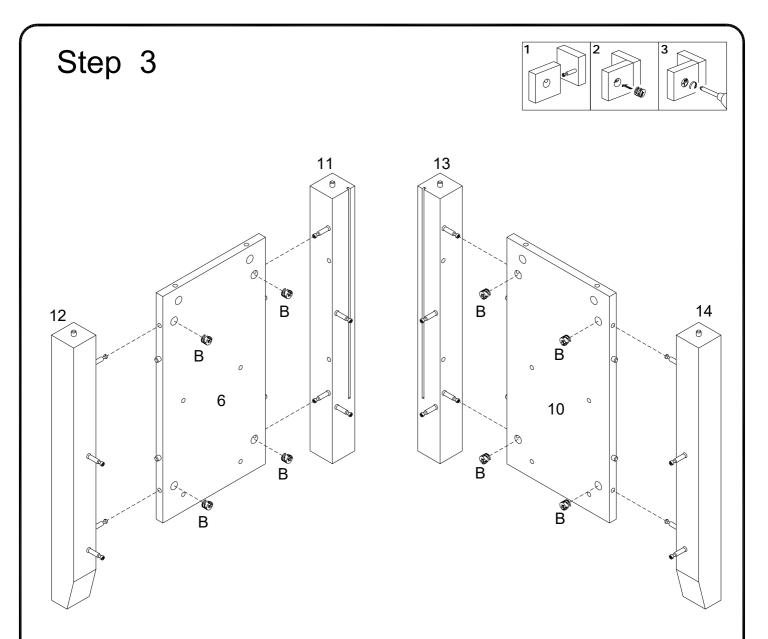
Using Cam lock(B) attach parts (11,12) to part (6) ,parts (13,14) to part (10) with Philips head screwdriver as per diagram.
