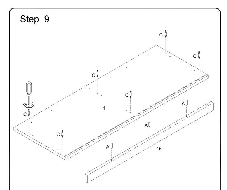
Insert wooden dowel (A) into part (15) ,then secure cam bolt (C) into part (1) with Philips head screwdriver as per diagram.
