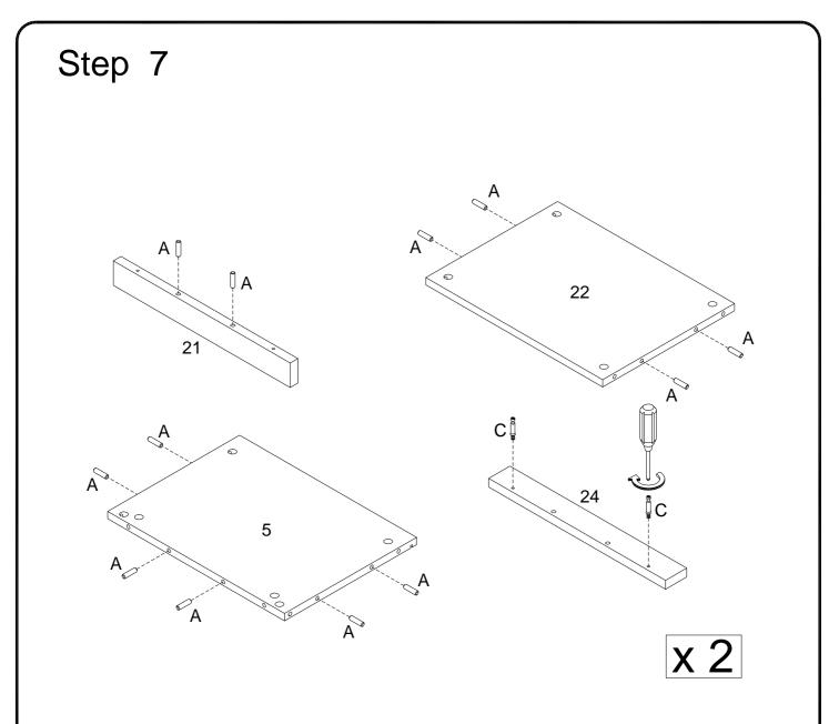
Insert wooden dowel (A) into parts (5,21,22) ,then secure cam bolt (C) into part (24) with Philips head screwdriver as per diagram.
