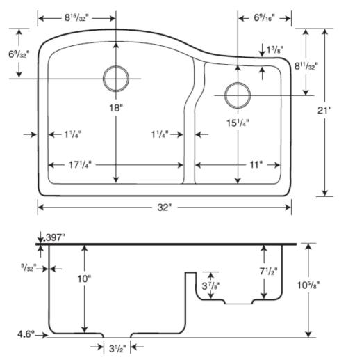
Capacity:  $8 \frac{1}{2}$  gallons in large (left) bowl until it reaches the divider height,  $2 \frac{1}{4}$  gallons in small (right) bowl until it reaches the divider height
