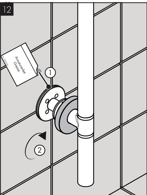
Lightly lubricate the o-ring on the bottom mounting plate using white plumbers grease.
