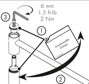
Lightly lubricate the o-ring on the top of the riser. Push the shower arm into place.
