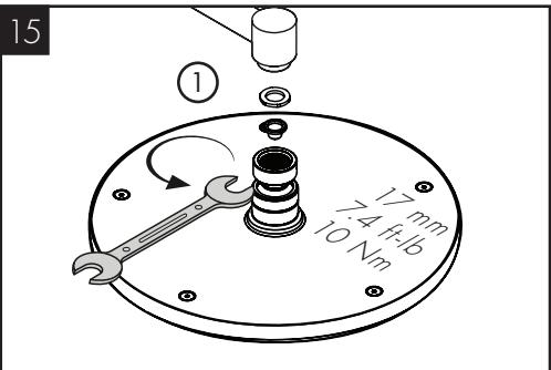
Install the showerhead with the filter and the washer.
