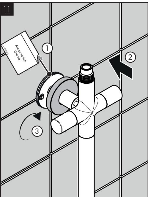
Lightly lubricate the o-ring on the top mounting plate using white plumbers grease.
