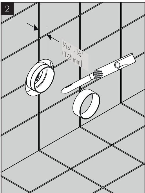
Cut the plaster shield so that it extends  $\frac{1}{16}''$  -  $\frac{1}{8}''$  (1 - 2mm) outside the surface of the finished wall.
