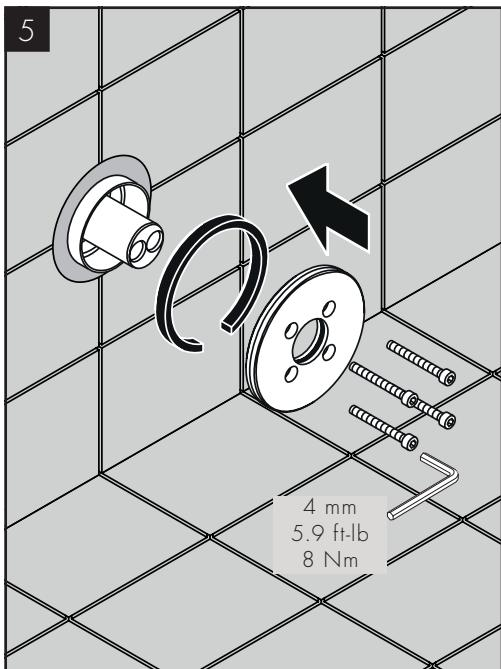
Install the mounting plate seal and the mounting plate.
