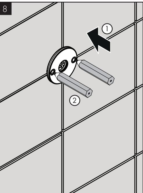
Place the top mounting piece against the wall at the marked location.
