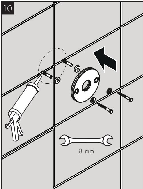
Install the anchors. Seal the wall around the anchors using waterproof sealant.
