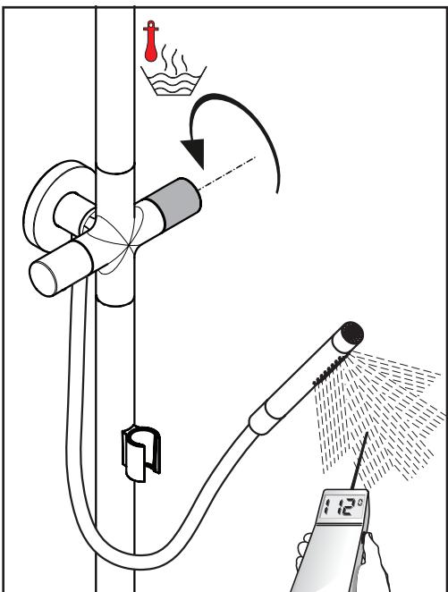
Turn the thermostatic mixer handle to the full hot position.
