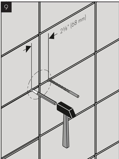
Drill the screw holes using a  $\frac{1}{4}$ " (6 mm) bit.
