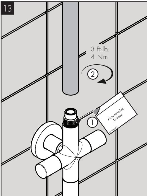
Lightly lubricate the o-ring on the top of the shower column.
