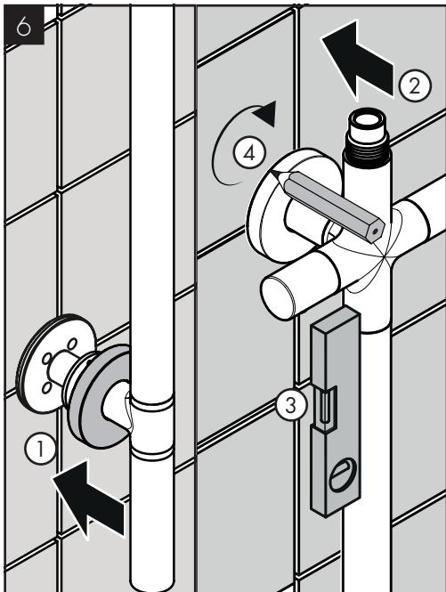
Push the bottom of the shower column over the seat and mounting piece.
