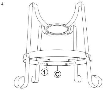
Loosely secure Large Ring (C) to the legs by hand-tightening four M6x8mm Bolts (1).
