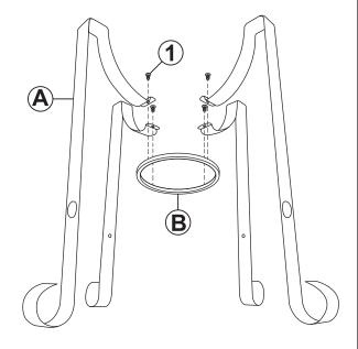
Align the holes in Small Ring (B) with the bottom of four Legs (A), as shown. Loosely attach the ring to the legs by hand-tightening four M6x8mm Bolts (1).
