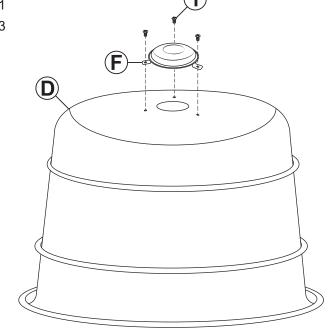
Securely fasten Ash Tray (F) to the bottom of Smokeless Fire-Bowl (D) using three M6x8mm Bolts (1).
