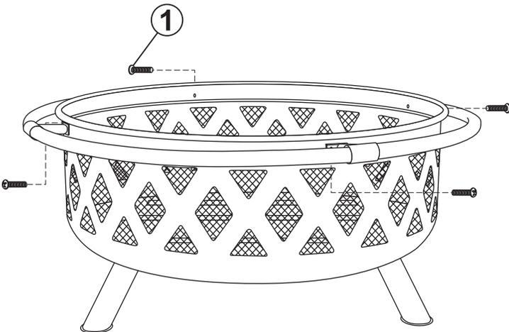
Carefully guide the assembled ring up from the bottom of the fire bowl, align the safety ring brackets with the mounting holes in the fire bowl, and loosely fasten it using four M6x25mm Bolts (1) and M6 Nuts (3).
