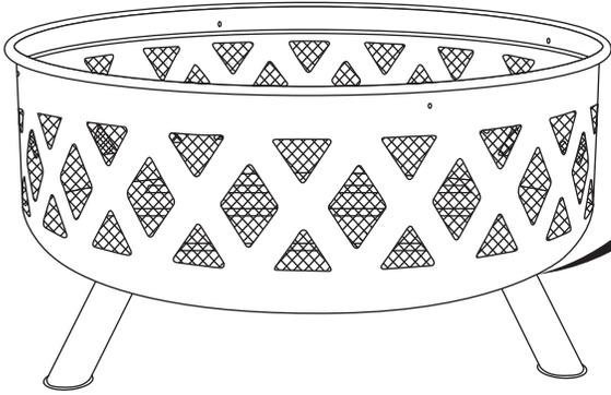
Ensuring the flat edge of the leg is facing outward, align Leg (B) with the bottom of Fire Bowl (A) and loosely fasten using three M6x10mm Bolts (2) and M6 Nuts (3).
