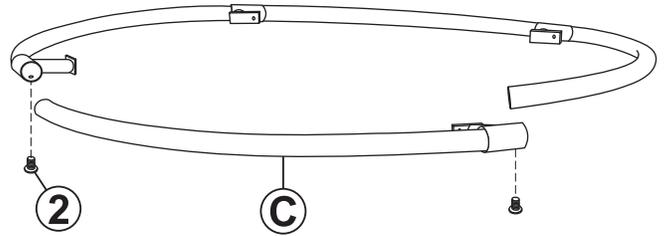
Align the mounting holes on the four Safety Rings (C) and loosely secure using four M6x10mm Bolts (2).
