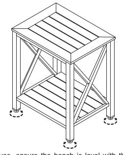
• Before use, ensure the bench is level with the floor. Turn the threaded feet until balance is achieved.
