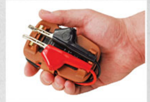
On-board test lead storage
