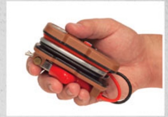
Test leads wrap around "racetrack" in Toner and snap securely in place
