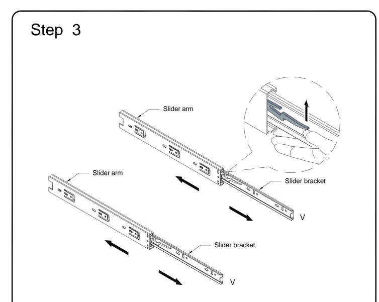
Pick up the slider arm (V) and separate the slide runner for the following Steps. Extend the slide runner all the way forward, press the plastic release lever of the slider arm up and pull the slide runner complete out .
