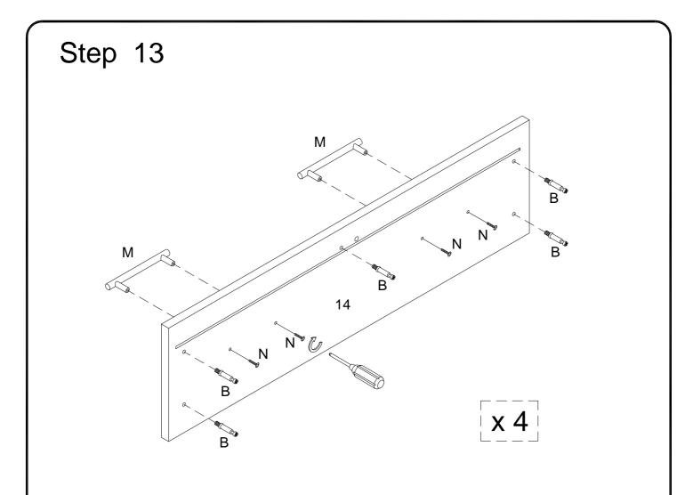
Secure cam bolt (B) into part (14) ,then using handle bolt (N) secure handle (M) to part (14) with Philips head screwdriver as per diagram.
