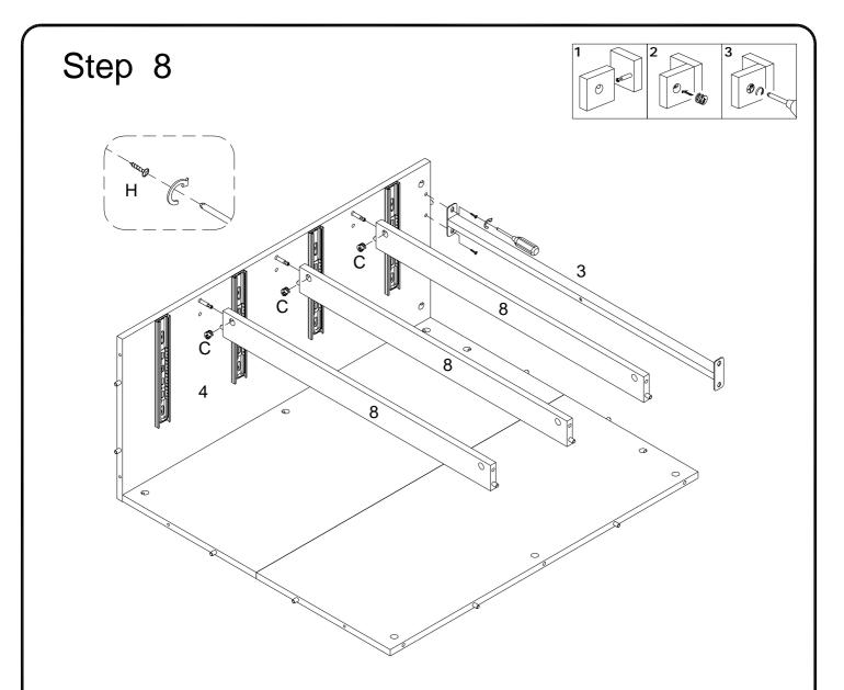
Using Cam lock(C) secure part (8) to part (4) ,then using screw (H) attach part (3) to part (4) with Philips head screwdriver as per diagram.
