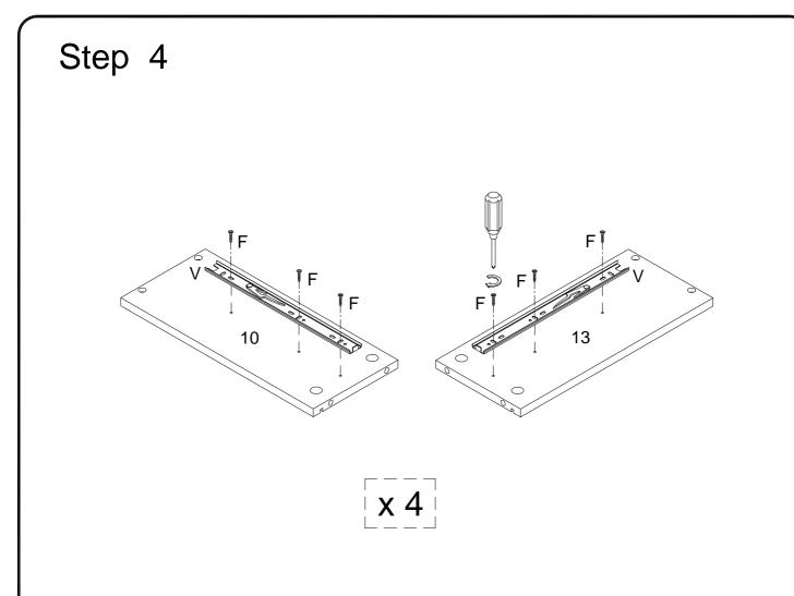
Using screw (F) attach drawer slider (V) into parts (10,13) with Philips head screwdriver as per diagram.
