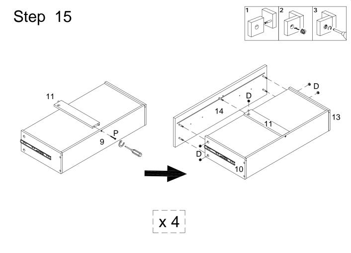
Using screw (P) attach part (11) to part (9), then using Cam lock (D) attach part (14) to parts (10,11,13) with Philips head screwdriver as per diagram.
