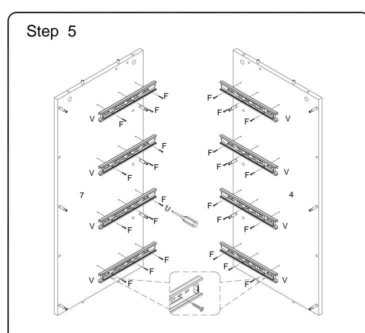
Using screw (F) attach drawer slider (V) into parts (4,7) with Philips head screwdriver as per diagram.
