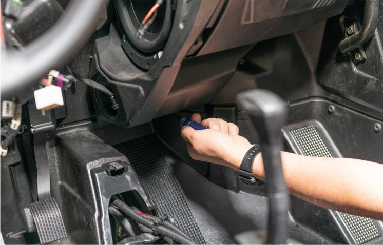
4. Feed the power and ground cables from the RZR-10A through the firewall grommet (Depending on model year, some tape may have to be removed from the grommet).
