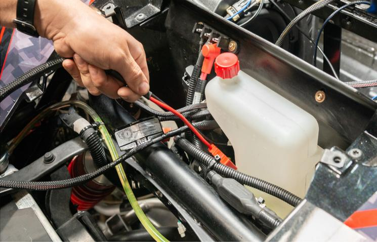
6. Feed the power and ground cables along the center of the vehicle along all factory wiring. Avoid any rotating parts or sharp edges when leading the cables to the battery.
