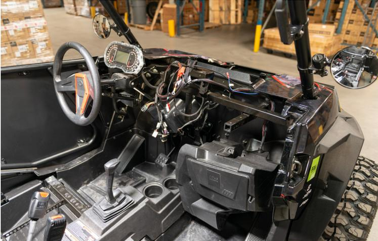
2. Lift the RZR-10A to the dash cavity crossbar. Secure the enclosure to the chassis with the factory 10mm hardware that was formally used to secure the glovebox to the machine.
