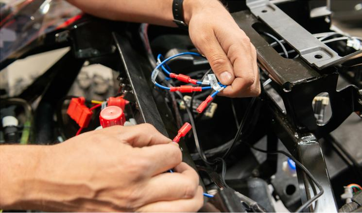
4. Replace the 12V socket with MUSB35, then tape off the power and ground to the 12V socket to prevent electrical short.
