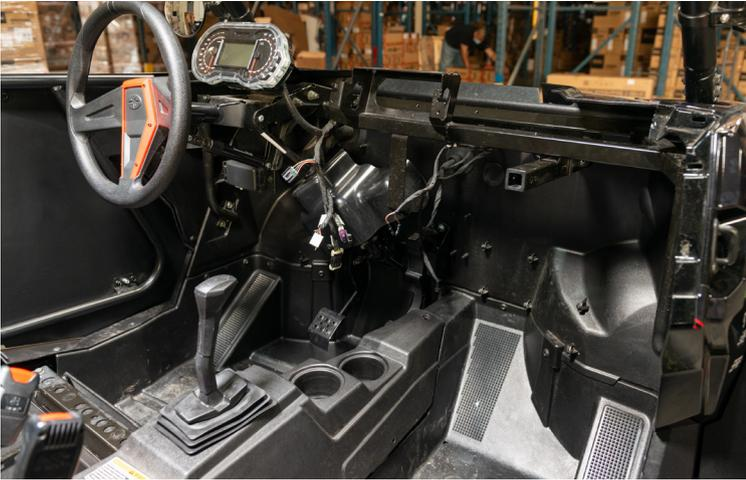
6. When removing the center console from a four-seat machine, disconnect the 12V socket found at the passenger rear of the center console.
