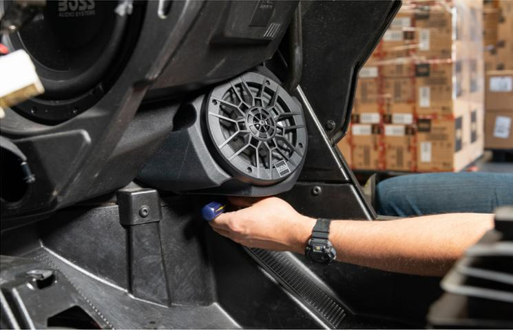
3. Using two of the provided #2 phillips screws, secure the inner two mounting points of the RZR-FSA to the firewall.
