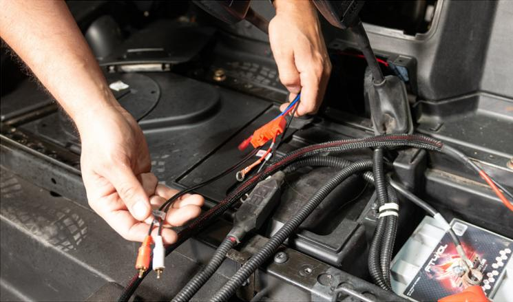
3. Route RZR-62A power, ground, RCA inputs, and remote turn on wire to the center console of the vehicle.
