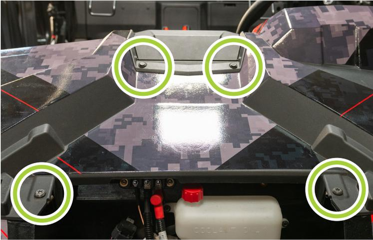
4. Remove the remaining push pins, T40 screws from the remaining dash components. Label takes photos/notes of all wiring that is connected to the dash face. Disconnect ignition, rocker switches, and 12V socket (from main dash face), and LED (lower storage compartment).
