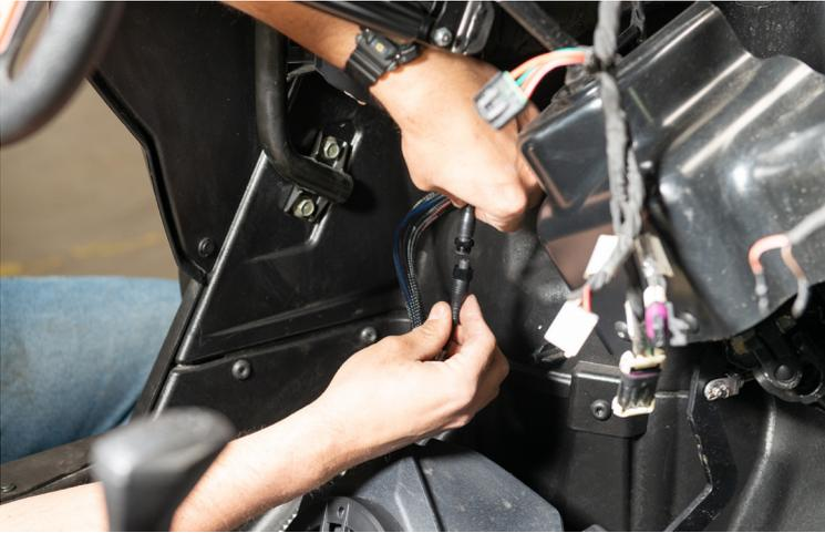
5. Reinstall one T40 Torx screw and fasten the two inner #2 Phillips screws.
