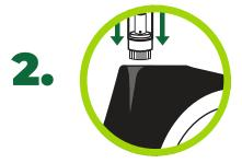
Drop cartridge with the magnetic adapter into the battery chamber.
