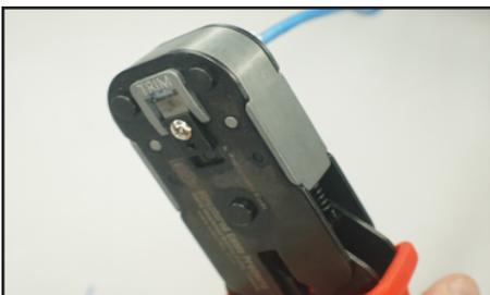
The Simply45 crimper is a ratcheted crimper. The crimper will not open up until the crimping process has been fully completed. This assures that the wire trims and pin sets have been done correctly.
