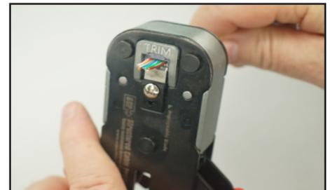
With one hand, firmly without stopping, compress the crimper handles all the way down in one steady non-stop motion.
