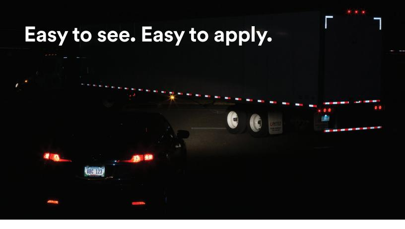
3M™ Diamond Grade™ Conspicuity Markings Series 983 are strong and rigid with a high performance adhesive that holds securely to vehicles. Markings are available in rolls, packaged pieces or kiss-cut pieces on a roll. The easy-release liner makes installation quick and user friendly.
