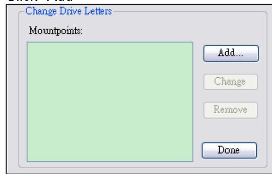
Assign a letter to the HDD, then click "OK" so that the HDD get a drive letter and can be recognized by Windows.
