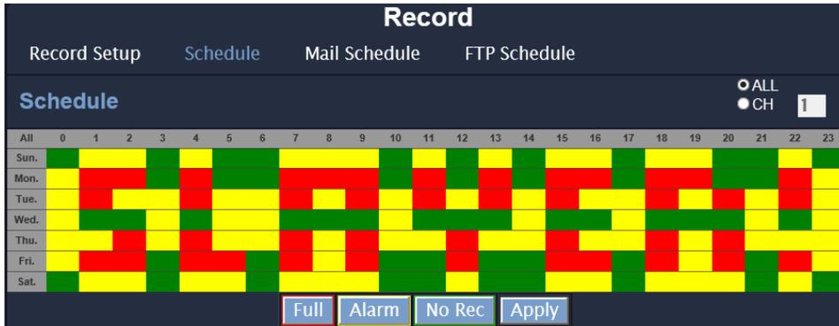
Click the tag **“FULL REC”**(Red) / **“ALARM REC”**(Yellow) / **“NO REC”**(Green), and then draw on the calendar. The recording type will follow the schedule. The tag **“ALARM REC”** includes all the alarm types.
