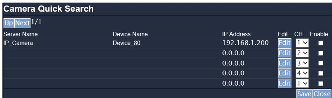
Back to the all-channel list, you can key-in the user name and password, and tick “Enable” to connect to the camera. If you want to revise the IP setting of a camera, click “Edit”:
