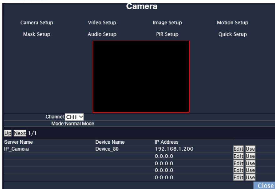
Click **IP Installer** to begin the search. The NVR will search for any network device in connection with the NVR. You can edit the IP address of the IP camera by clicking **Edit** icon.
