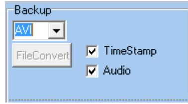
After double-clicking on one specific channel display image, the 'File Convert' button will be available. Select the type of video format you would like to convert to from the Backup drop down list.
