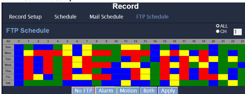
Select the time that the recording video is uploaded to FTP. No file will be uploaded during “**NO MAIL**” period even the motion detection is triggered. The tag “**ALARM FTP**” refers to both external alarm and DI from camera.
