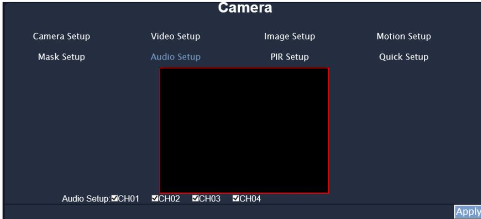
The channel ticked means the sound from the network camera will be recorded into the playback video. On the contrary, no sound will be recorded in playback video for the channel not ticked.
