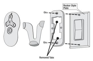
**Note:** For rocker-style cover plates, break off the tabs by pushing outward.
