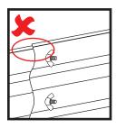
Do not fully tighten hardware until all components have been loosely assembled.
