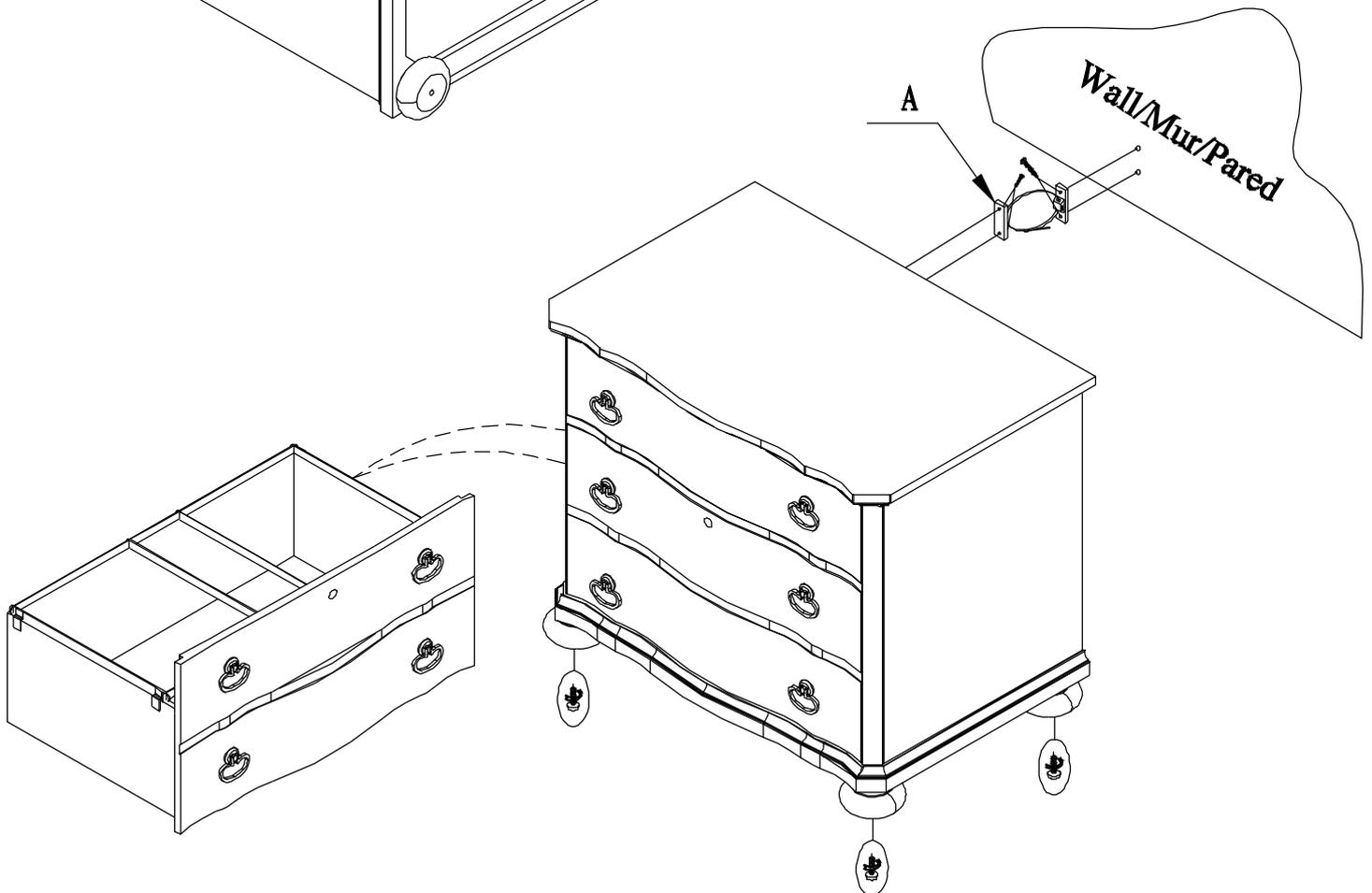
**Adjust levelers if needed, to level case on uneven floor**
