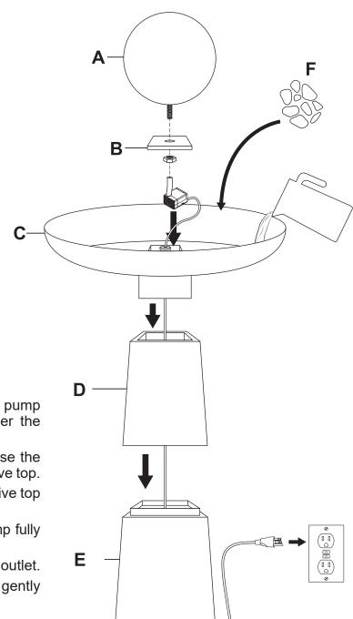
NOTE: When first plugged in, there may be air trapped in the pump. It may take several moments for trapped air to escape, allowing water to flow.
