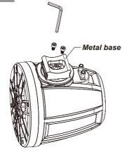
To adjust the mounting angle, loosen the metal base of the mounting band by unbolting the two screws.
