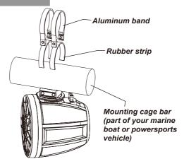
Place a supplied rubber strip around the cage bar to prevent abrasion and secure clamping. Then push two supplied aluminum bands over the cage bar, and align the aluminum bands with the metal base on the speakers.
