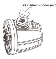
Place a supplied rubber (49 x 40 mm) pad on the metal base of the mounting band to prevent abrasion and secure clamping.
