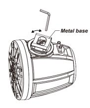
Twist the metal base to determine the optimal mounting angle for the speaker on the cage bar. Then secure the metal base by tightening the two screws.
