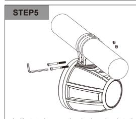
As illustrated, secure the aluminum bands to the metal base using a pair of M6 x 75mm screws, M6 flat washers, and M6 locknuts. The locknuts must be installed into the hex shaped recess on one end of each aluminum band.
