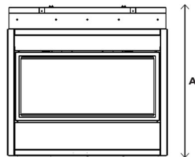
\*Finishing flange depth (The finishing flange defines the perimeter of the fireplace opening). Framing or finishing materials must NEVER encroach inside the finishing flange.
