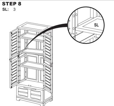
Insert Shelf (SL) into the unit at a slight angle and align the shelf with one side of the unit. Then, gently press on the opposite side of the shelf until the shelf locks into place.
