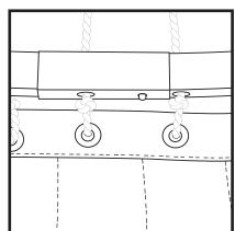
Push the bars together until the spring button snaps through the hole in the metal bracket.
