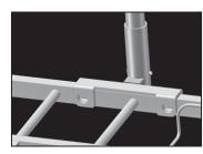
3. Re-insert the metal pins through the mounting holes and secure with the snap rings. Make sure the snap rings are positioned in the groove of the metal pins. Repeat the same procedure to install the other rail.
