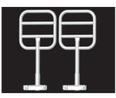
2. Unclip and remove the metal pins from the rail mounting brackets. Hook the rail bracket onto the edge of the bed decking. Align the rail bracket mounting holes with the bed decking mounting holes.
