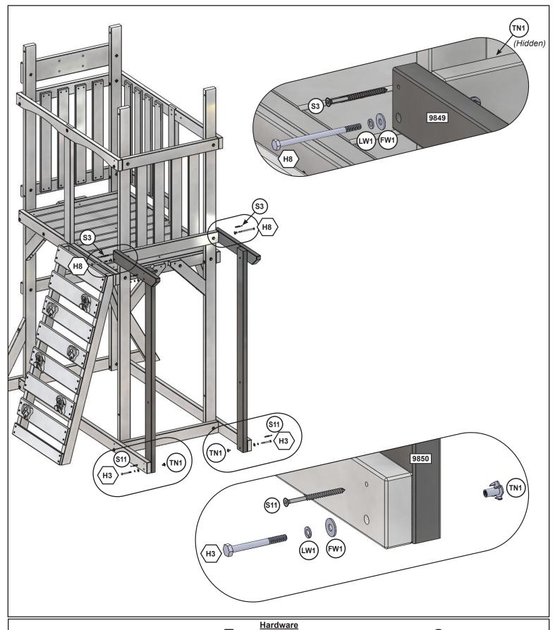
2 x  $\langle H3 \rangle$  6.4 x  $\overline{63.5}$  mm (1/4 x 2-1/2") (FW1, LW1, TN1) 2 x  $\langle H8 \rangle$  6.4 x 108 mm (1/4 x 4-1/4") (FW1, LW1, TN1) 2 x (S11) #8 x 50.8 mm (#8 x 2")
