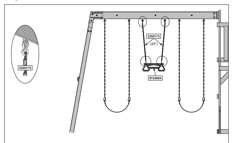
Caution: Threaded Quick Links must be installed with the gate completely down covering the threads and tighten as instructed.
