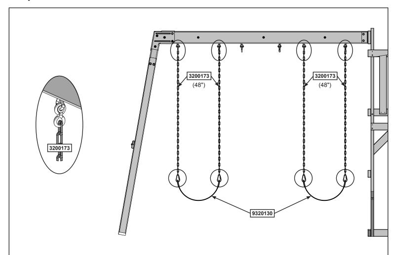
Caution: Threaded Quick Links must be installed with the gate completely down covering the threads and tighten as instructed.
