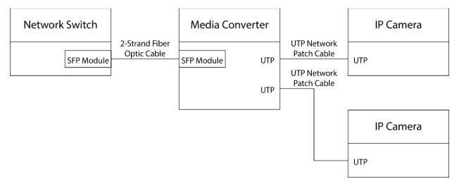
Example 2 - extend LAN signal using switch without SFP ports.
