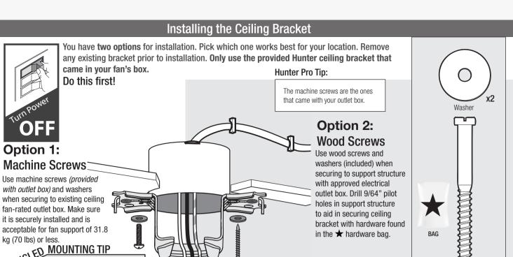
To avoid possible electrical shock, before installing your fan, disconnect the power by turning off the circuit breakers to the outlet
