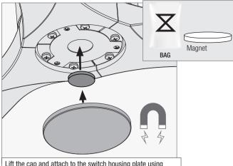
Lift the cap and attach to the switch housing plate using magnet found in hardware bag X. Cap will snap to place magnetically.
