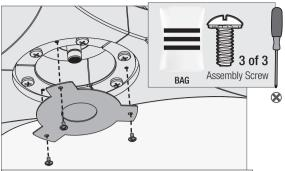
Lift the lower switch housing until its screw holes are aligned with the screw holes in the blade irons. Install the three assembly screws, found in the hardware bag = . Tighten all three screws.
