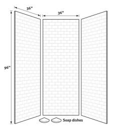
Designed to fit base areas 36" deep or smaller x 36" wide x 96" high or smaller (914 mm x 914 mm x 2438 mm)
