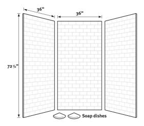
Designed to fit base areas 36" deep or smaller x 36" wide x 72-1/2" high or smaller (914 mm x 914 mm x 1829 mm)
