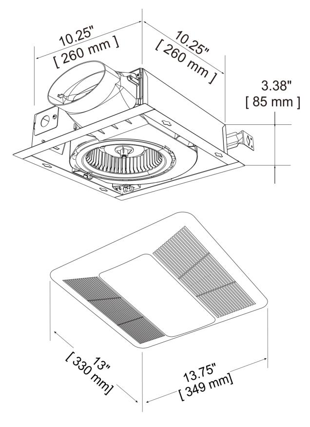
This fan can be installed to 10.5" - 21" between the joist or to I-joists, standard joists and truss construction.
