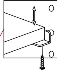
The adjustable shelf is screwed in place to avoid damage during transit.
