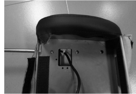
STEP 7: Slide on the edges of the leather cover from left to right.
