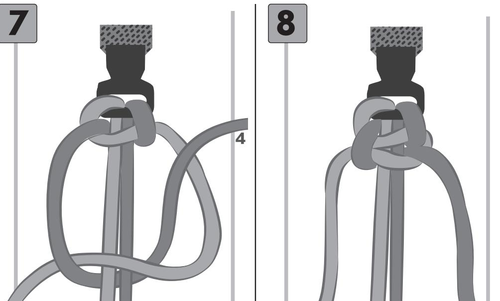
Pass the left cord (4) under the two center cords (2 and 3) and up through the loop you made on the right.
