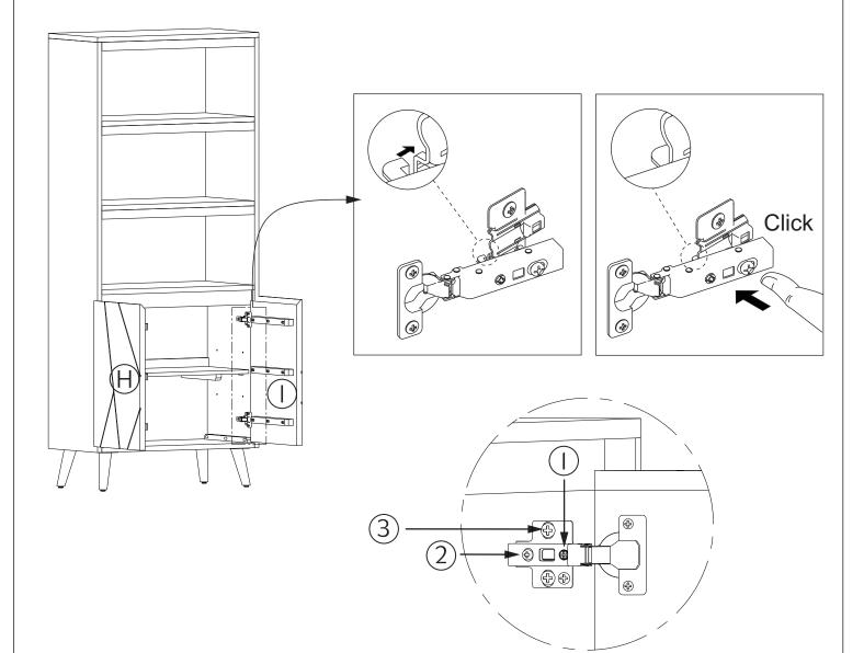
Attach Door Panels (H) and (I) using adjustable hinges on Side Panels (A) and (B).
