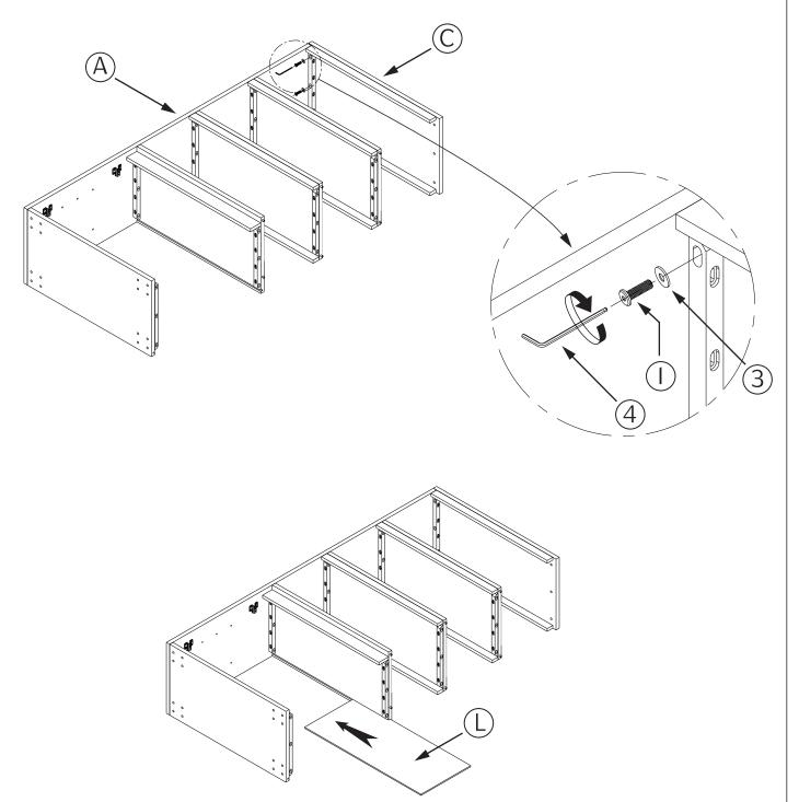
I. Align holes on Top Panel  $\bigcirc$  with holes on Left Side Panel  $\bigcirc$ .
