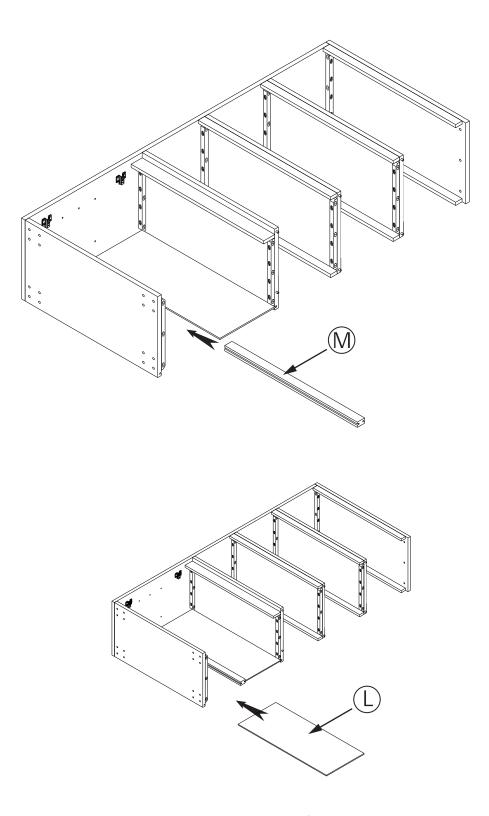
I. Insert Back Connector M and second Back Panel L.
