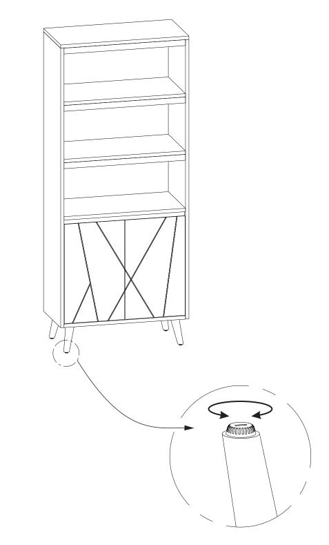
Note: Levelers on bottom of legs can be adjusted if floor is uneven.
