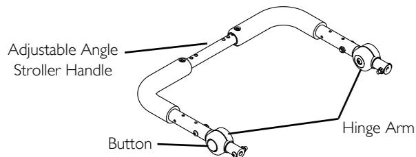
**FIGURE 5** Adjusting the Adjustable Angle Stroller Handles
