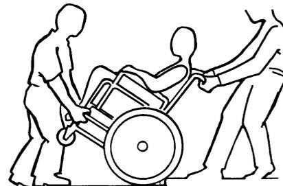
**FIGURE 4** Tipping - Curbs: Method 2 - Wheelchair without Step Tube
