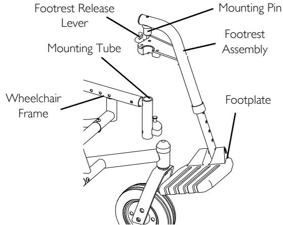
**FIGURE 1** Installing/Removing Footrests
