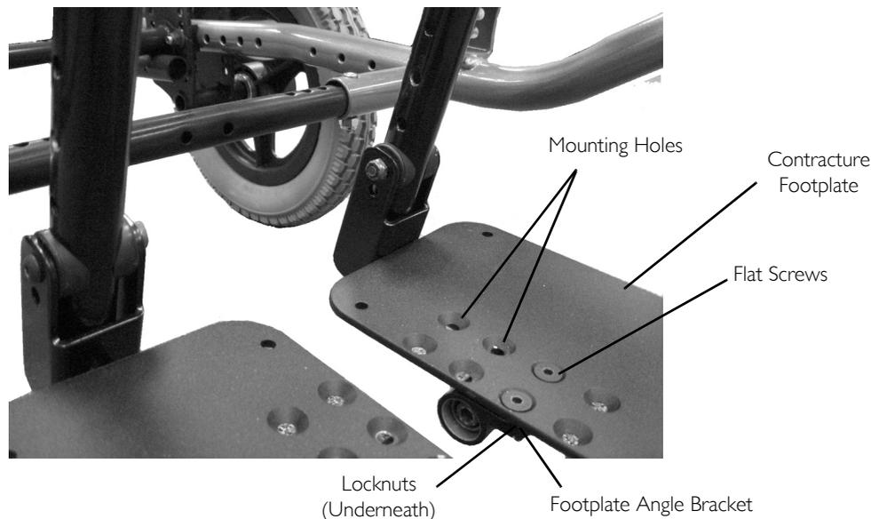
**FIGURE 4** Depth Adjustment - Bilateral Contracture Footplate
