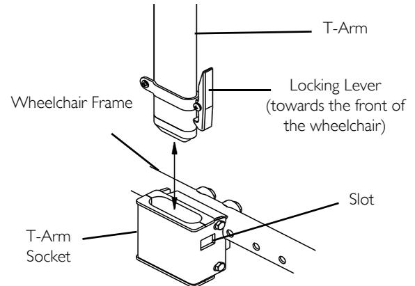
**FIGURE 7** Installing/Removing T-Arms
