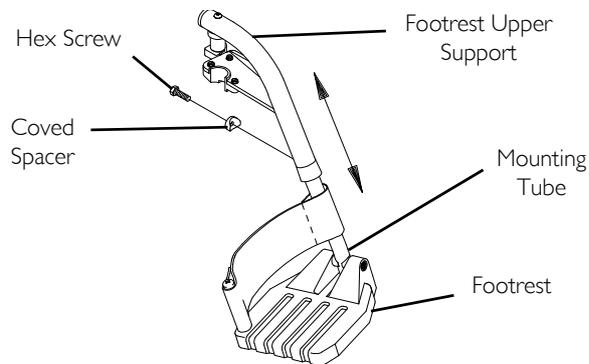
FIGURE I Adjusting Footrest Height - 60°, 70° and 70° Taper
