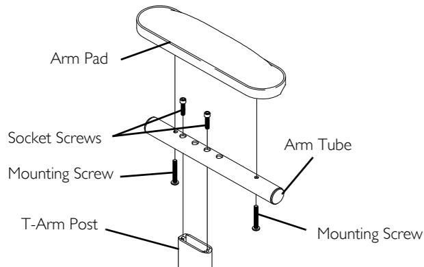
**FIGURE 4** Adjusting T-Arm Depth
