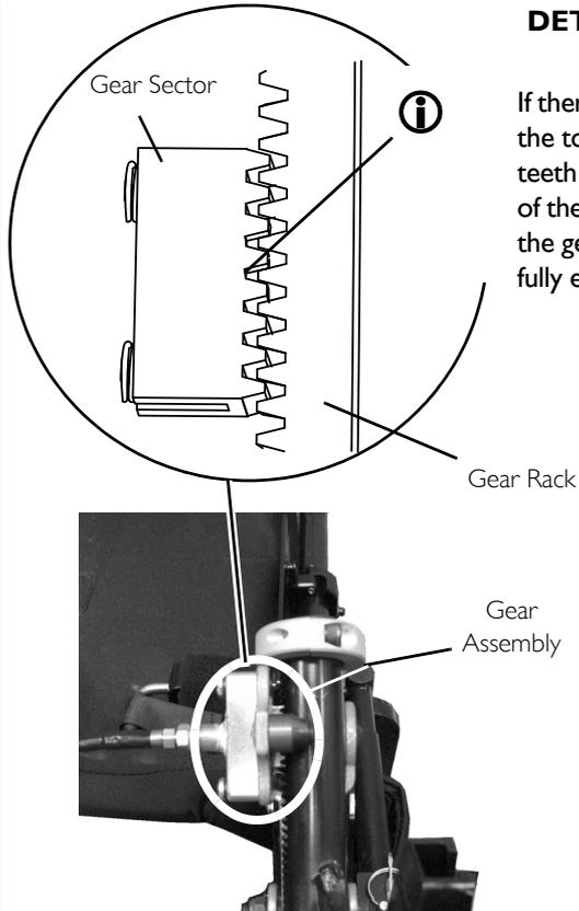
**FIGURE I** Adjusting Tilt-In-Space Trigger Release Cables
