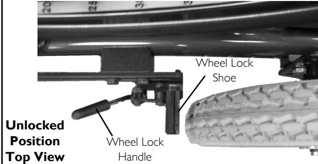
**FIGURE 10** Using the Pull to Lock Wheel Locks
