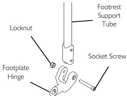
**FIGURE 3** Installing Adjustable Angle Flip-Up Footplate Hinge
