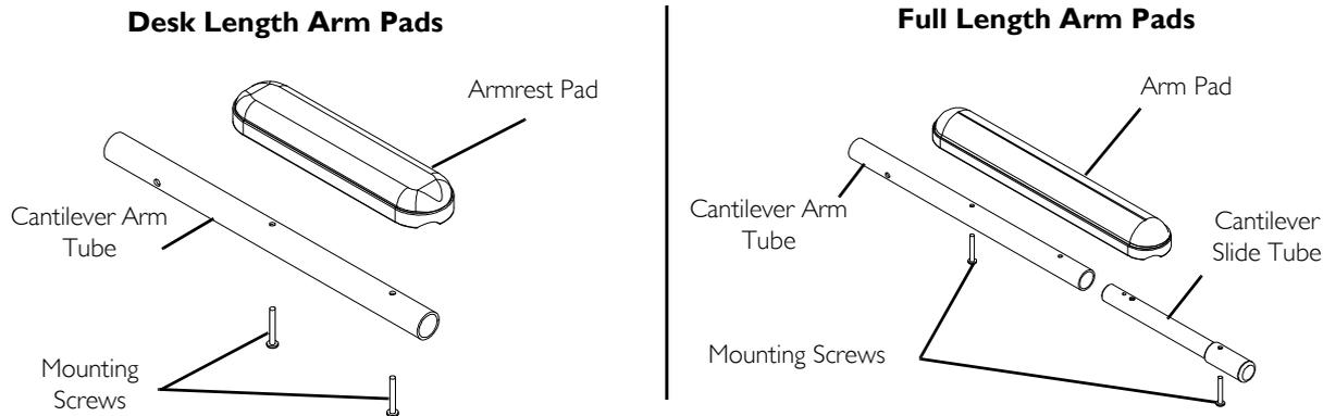
**FIGURE 11** Arm Pad Replacement for Cantilever Arms
