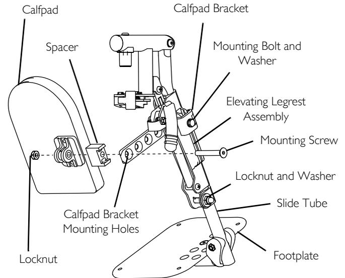
**FIGURE 6** Adjusting Footplate Height and Calfpad Height/Depth
