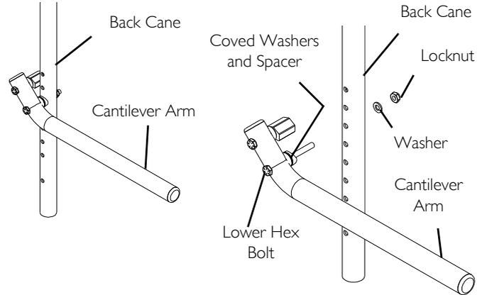
**FIGURE 9** Installing Non-Locking Cantilever Arms
