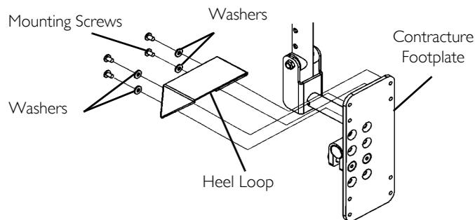
**FIGURE 8** Replacing the Contracture Footplate Heel Loop
