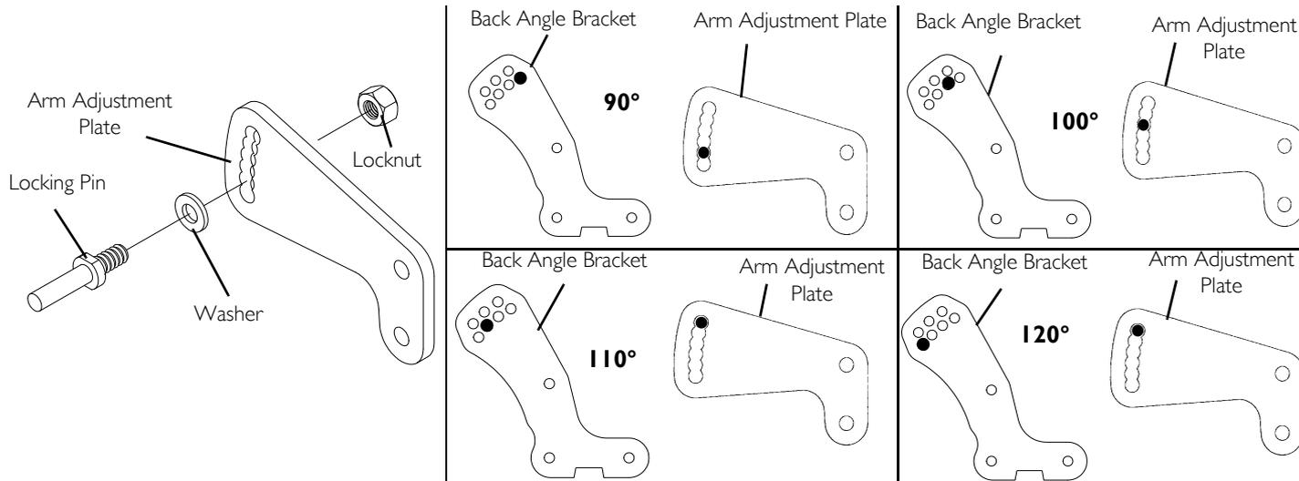
**FIGURE 8** Adjusting the Locking Cantilever Arm Angle
