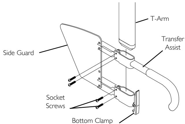
**FIGURE 6** Adjusting T-Arm Transfer Assists And/or Side Guards.
