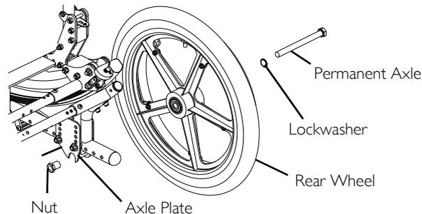
**FIGURE 14.1** Installing/Removing Rear Wheels - Permanent Axle
