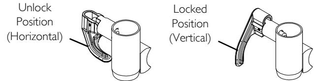
**FIGURE 5** Removing/Installing Flip Back Armrest
