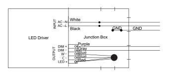
Reattach cover of junction box and secure with screw. To adjust CCT or Lumen output, set the switch positions on the side of the driver to the desired settings.
