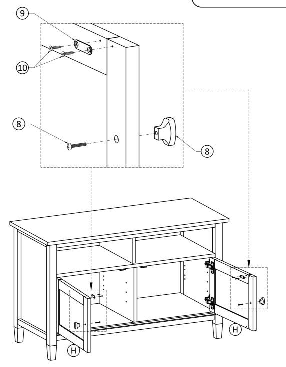
1. Attach Magnet Plates (9) using Phillips Screws (10) into pre-drilled holes on Doors (H).
