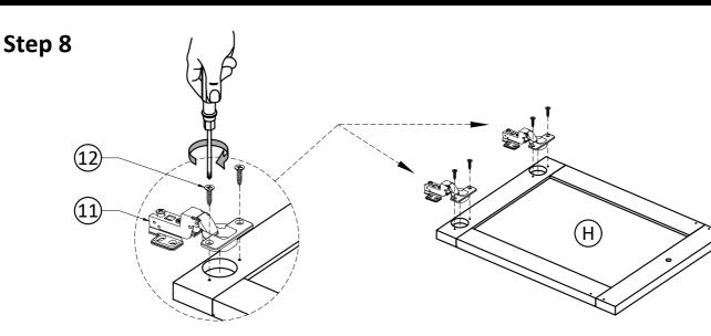
1. Attach Adjustable Hinges 11 to Doors (H) using Phillips Screws (12) into pre-drilled holes on Doors (H).
