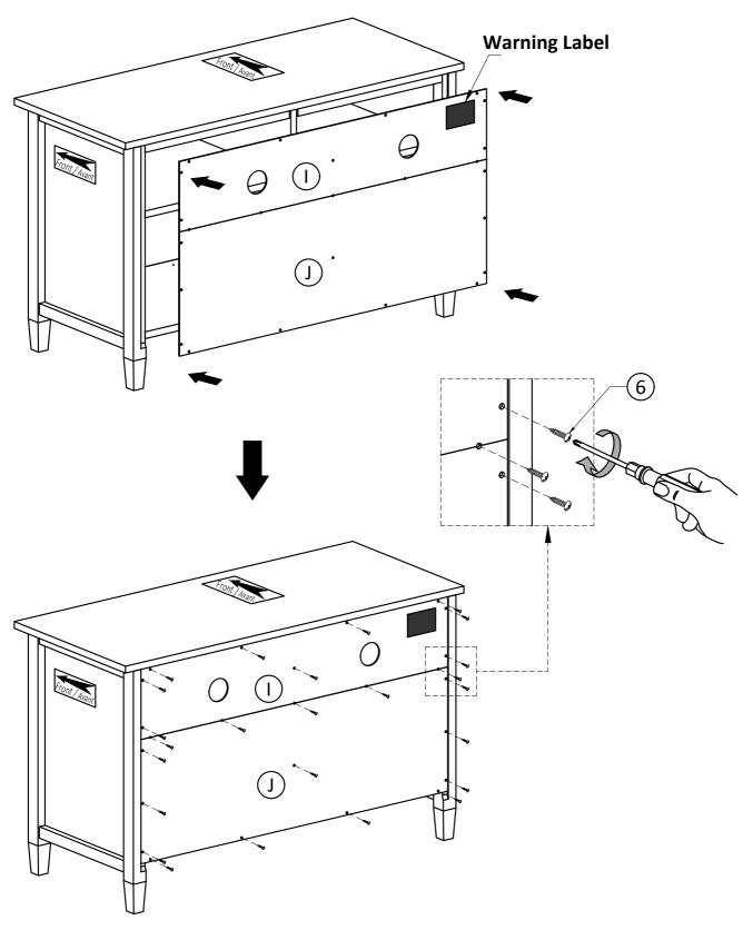
Attach Back Panels (1), (1) to back frame by using Phillips Screws Round Head (6).
