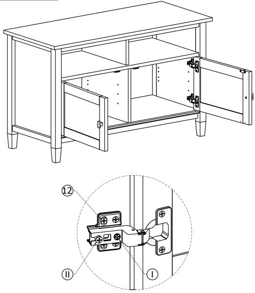
Tighten the Screw marked (II) to fasten hinge. The door may need to be adjusted so that all the spaces between the door and the unit sides are equal. To adjust, follow instructions:
