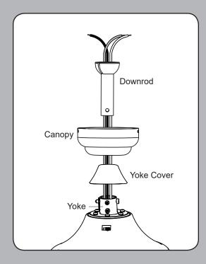
2. Feed the wires through the yoke cover, canopy, and downrod.
