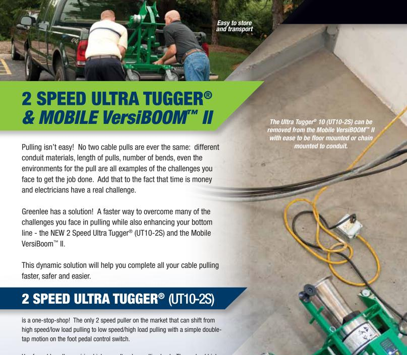
Use for cable pulls requiring high as well as low pulling loads. The no-load high speed is 16 ft./min. and is best suited for loads up to 4,000 lbs. where the speed will be 12 ft./min. The no-load low speed is 9 ft./min. and can be used on loads up to 8,000 lbs. where the speed will be 6 ft./min., or a momentary peak capacity of 10,000 lbs.
